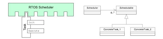
It is concluded that in an AOCS there is at least one functionality – task scheduling – where a framework approach improves reusability. Task scheduling is only one of many functionalities implemented by an AOCS and it is natural to ask whether the same principles that make it reusable could be applied to the other AOCS functionalities. The chief achievement of the AOCS project was to show that this is indeed possible.
